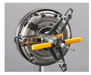
Example installation: travel-controlled self-adjusting clutch
