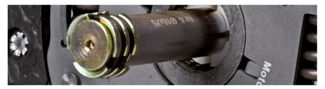
Correct assembly of the centring pin is dependent on the inner diameter of the pilot bearing or crankshaft bore, and on the distance between the pilot bearing or crankshaft bore and the clutch disc's hub profile.
