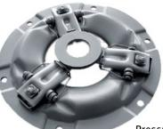
Pressure plate of an early diaphragm spring clutch
