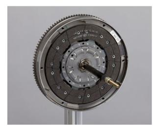
• Remove the centring pin along with the clutch disc.
