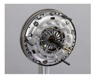
• When the diaphragm spring is completely relieved, remove the knurled nuts and pressure piece.
