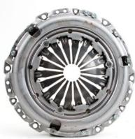
Pressure plate of a standard diaphragm spring clutch
