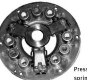
Pressure plate of a coil spring clutch
