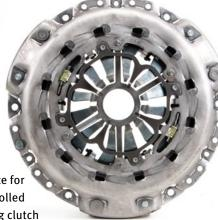
Pressure plate for a force-controlled self-adjusting clutch Pressure plate of a travel-controlled self-adjusting clutch
